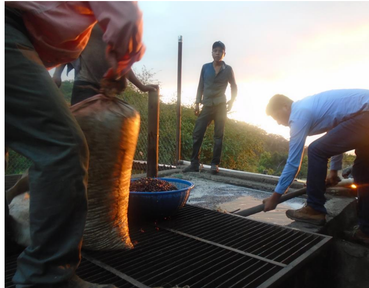
Skimming floaters off the density separation tank is highlighted by the setting sun
